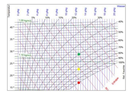
The diagram shows three air states that can occur at the same time in an apartment. The water content in the air is always approx. 12.5 g/kg, as the air flows through the entire usage unit.
