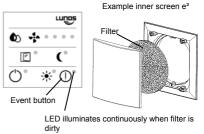
Please note the filter replacements you have carried out. (Filters should be changed approx. 3 months after the last filter replacement):
