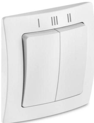
A total of 4 ventilation levels can be selected by pressing the rocker switches. If, as shown in the illustration, both rocker switches are set to the bottom, level 0 is active. This means that the fans run permanently at a very low level or are switched off (depending on the control setting). The so-called humidity control is an exception.
